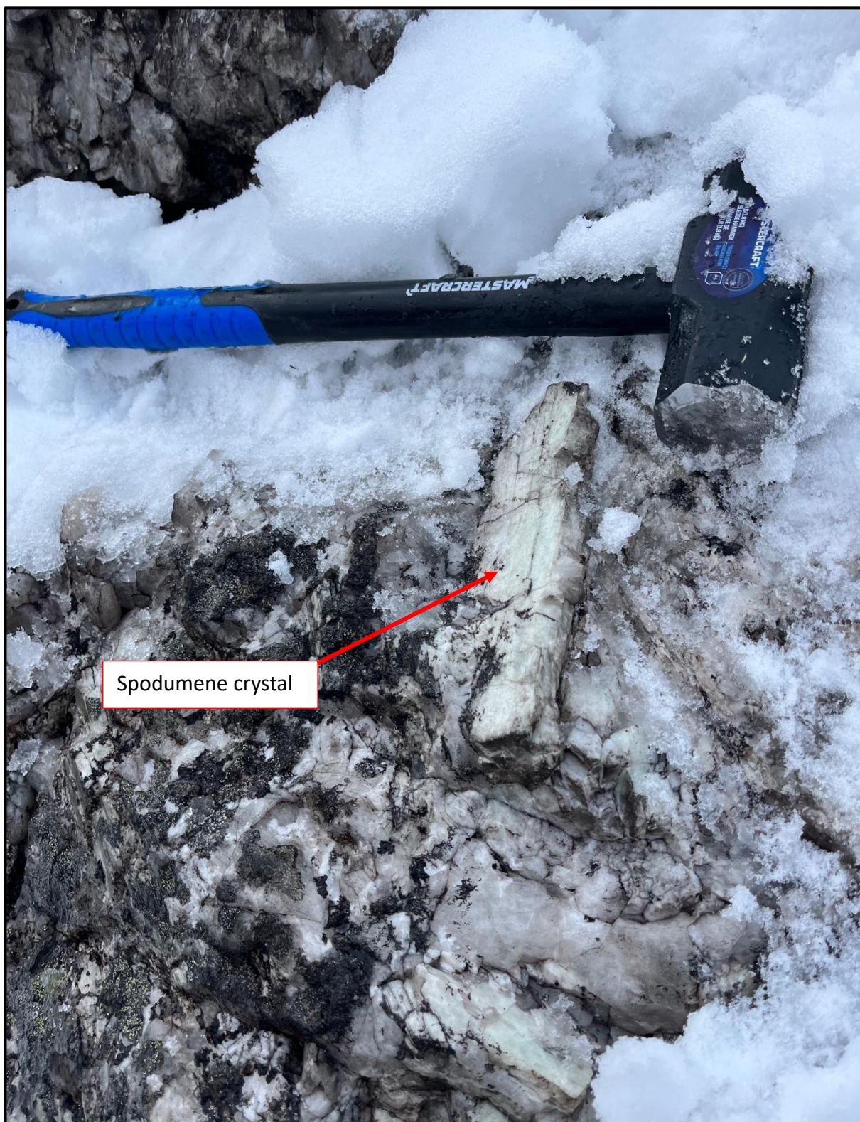
Figure 2. Photograph of the lithium bearing pegmatite sampled during the field work. Hammer is approximately 40 cm long for scale.
